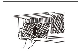
4. Remove the Air Freshening Filter from its support frame (on some models). (The optional filter include :Plasma Dust Collector/ Silver Ion filter /Bio filter /Vitamin C filter/3M air purifier filter, etc. The removing and installation methods are slightly different, see the pictures marked ① and ② on the left.
